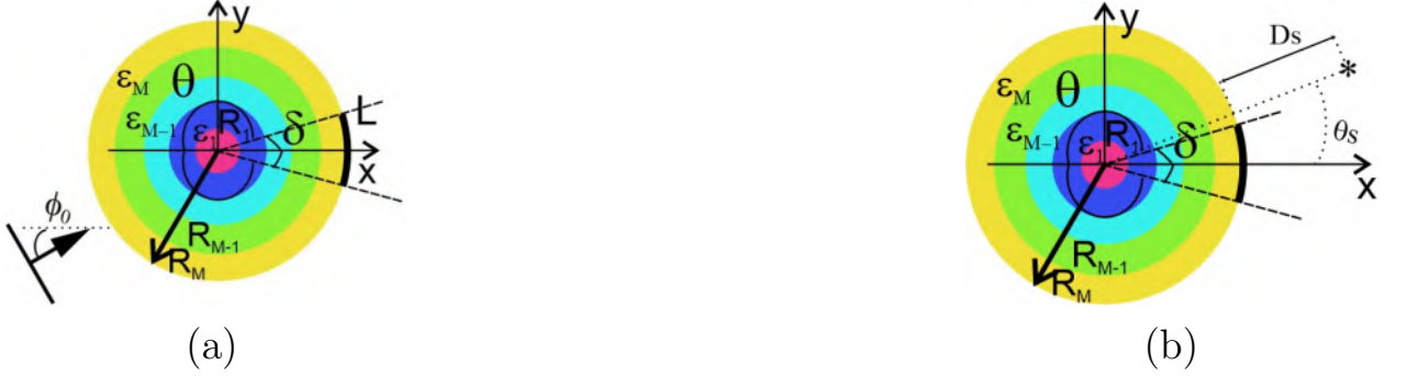
Figure 1.1: Cross sections of the bare discrete M -layer concentric Luneburg lens decorated with a conformal strip of graphene illuminated by the plane wave (a) and excited by the-point source (b). The strip is shown as a black arc centered at \phi = 0 .
